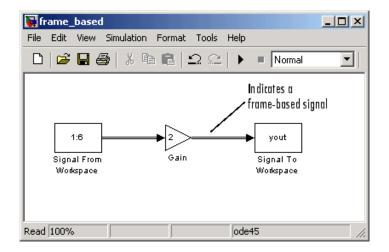
To have the Signal From Workspace block output a frame-based signal, set the **Samples per frame** parameter to 2 and run the model. The lines that connect the blocks become double lines, indicating a frame-based signal; in this example, there are two signals per frame.
